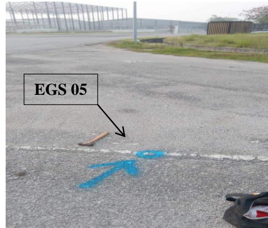
EGS05: E-45718.100, N-29028.135 (Nail embedded on road, painted blue)
